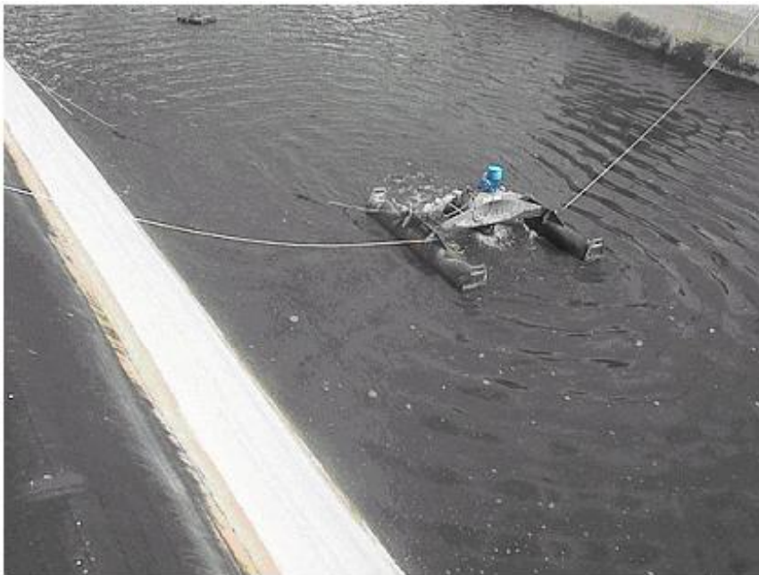
This is the situation eight weeks after installing the VitaOloïd and six weeks after installing the VitaFloat: a water storage basin without algae, with an oxygen level of 100%. Temperature, EC and pH are also the same throughout the whole basin
